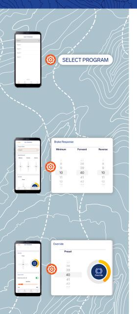
Your EB2 comes with default brake settings. We recommend adjusting your brake response to your specific requirements. To adjust the **minimum**, **forward**, **reverse** and **manual override** response, tap 'Settings' on the app.
