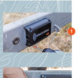
Fasten the EB2 to the drawbar using the mounting screws provided. For optimal SwayControl performance, mount your Elecbrakes EB2 within 1m of the tow ball.
