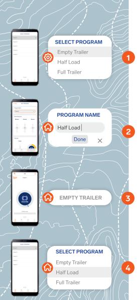
You must be connected to the brake controller to select and configure programs. Navigate to the 'Settings' page and select the program you wish to edit.
