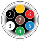
7 Pin Socket Cable entry view
